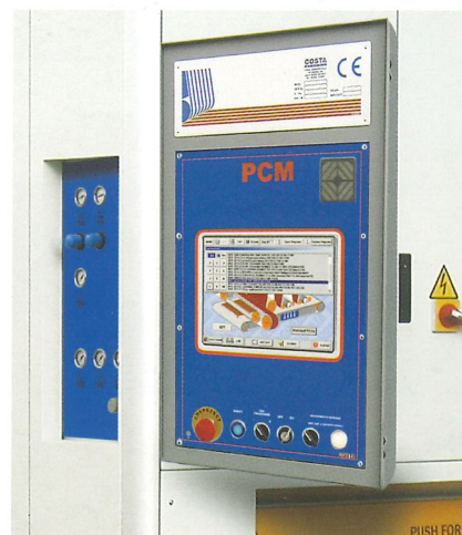
Possibility to have a 45° inclined panel board very usefull for machines positioned in line
