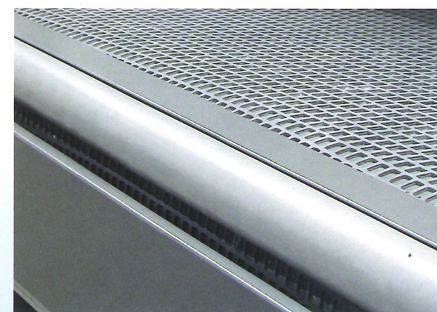
Machine infeed view with driven roller for line connection. (OPTIONAL)
