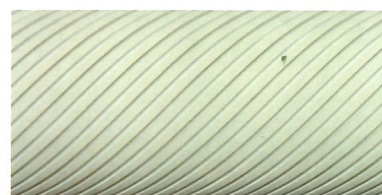
Special type of helicoïdal grooves on the surface of the cylinders for cooling and for air discharge
