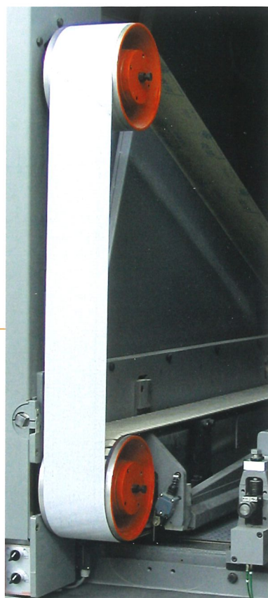
Dust hood in opposite side of internal cross belt unit (TRI),turnable 90° to easy the change of sanding belt.
