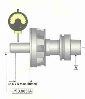
By combining two HSK interfaces, the Aerotech System® is able to guarantee maximum precision, concentricity and balance. Each Aerotech component is dynamically balanced to G2.5 at 25.000 rpm. Users are able to remove and replace the HSK 20C inserts independently by using the simple Aerotech demount device provided.
