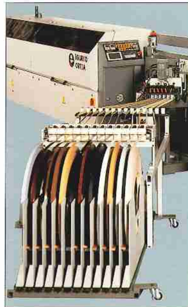
ALMACEN DOCE ROLLOS. 12 COIL MAGAZINE. MAGASIN 12 BOBINES. 12 ROLLEN-MAGAZIN.
