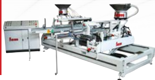
Foratrice incollaspine Boring and dowel inserting machine
