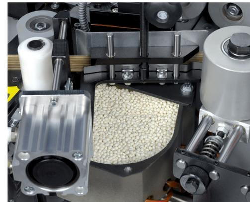
The 1.2 kg teflon coated glue pot is designed for EVA granulate glue. The glue is applied via an adjustable glue roller.
