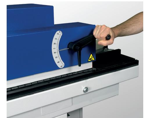
The height of the top pressure bar can be adjusted by a lever. This can be read easily thanks to a large scale.
