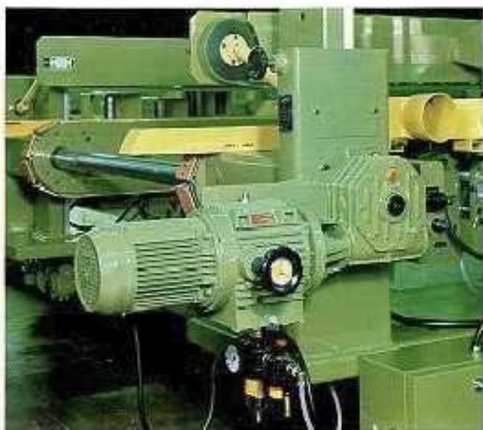
Track motor with hydraulic speed variator
