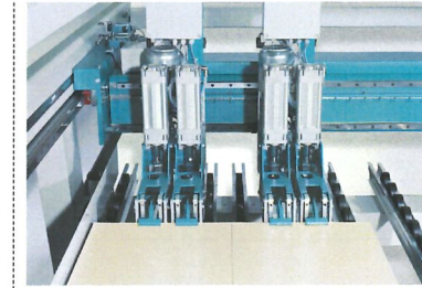
GIBEN PX-SP equipped with two couples of moving grippers along the length axis (X) of the pusher.
