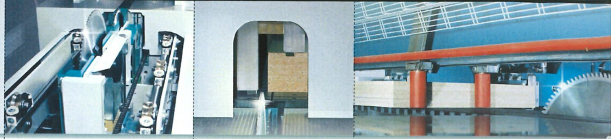
Saw carriage and "triangle shaped" guiding system.
