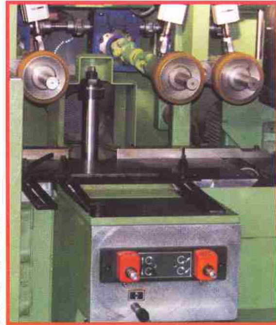
Toupies empilables (270 mm) Stacktooling spindle (270 mm) Hubspindel (270 mm) Tupi empilable (270 mm)
