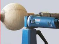
Upper tool bracket with diameter 43mm can be used also for routers
