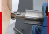
Tool-holder with HSS-cup-cutter for final cutting, fast change by 180° turning of the bracket, chiplimiter screw for safety reasons
