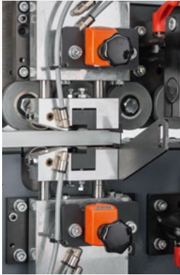
Surface scraper with dual-tracing
