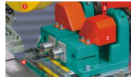
Saw Station 1. Infeed table with clamping units
