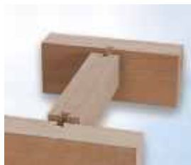
Components cut to length. Slots for Hoffmann Keys are routed. Where appropriate, dowel holes are drilled (with template or routing and drilling machine)
