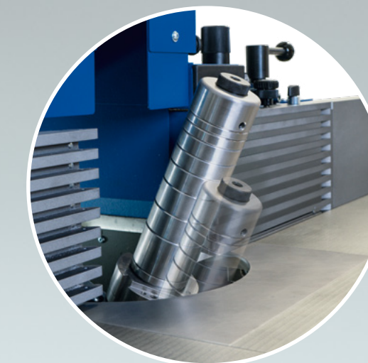
Height adjustment takes place linearly via the spindle
