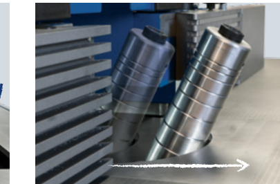
The depth is adjusted using the spindle, not the milling stop
