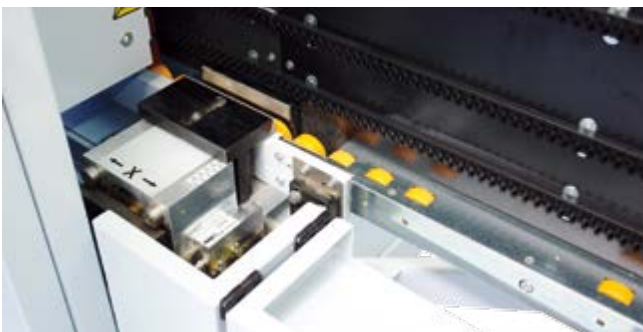
Workpiece clamping device Easy adjustment of the clamping device (manually) to the workpiece thickness (clamping device stroke 10 mm). For differences in the workpiece thickness of up to 10 mm it is not necessary to manually adjust the clamping device.
