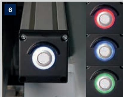
**Button for program start** directly on the left and right stop profile of the machine table. The clamping status is immediately in view thanks to the multi-colored light display.
