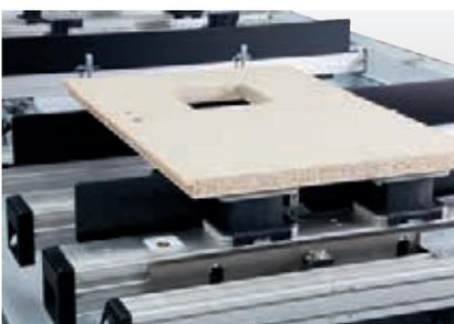
**Linear guide and insertion aid** – easy handling by consoles with highly precise linear guides and robust insertion aids with two pneumatic cylinders. Vacuum and compressed air connections for pneumatic clamps and clamping templates are integrated in the consoles.
