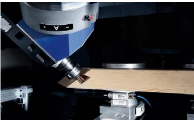
Routing a burr connection for jamb/rail designs
