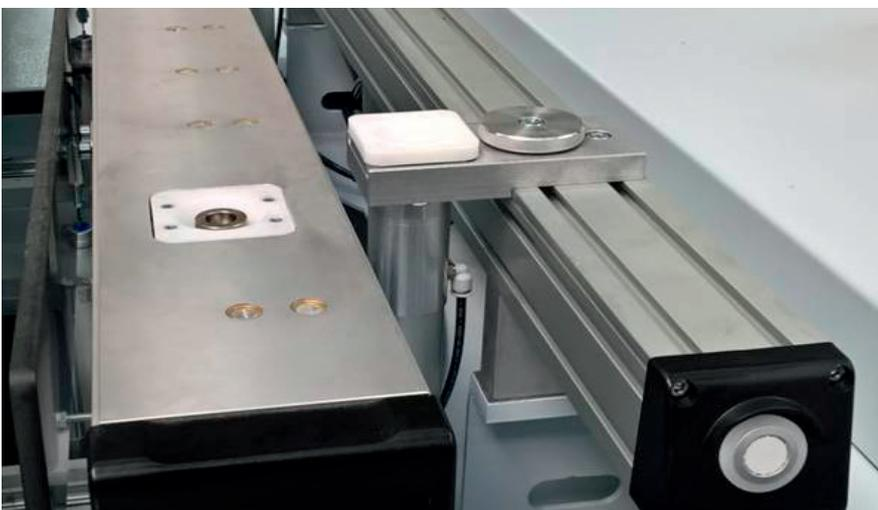
Side stops can be moved via a quickrelease mechanism.
