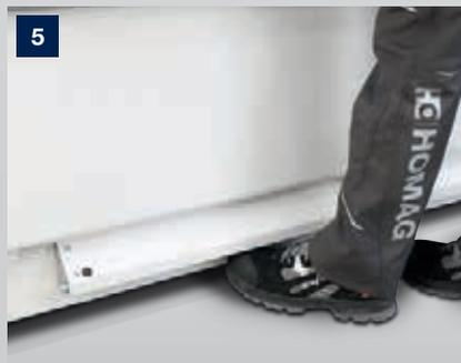
**Switch bar instead of foot switch** – no searching and moving the foot switch – stops, output stroke rails and vacuum clamping can be activated easily.
