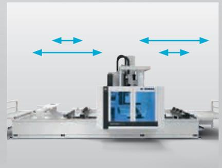
**Dynamic alternating operation** without fixed field subdivision. This means that even in the case of long parts on one side of the machine a short part can still be placed on the other side.
