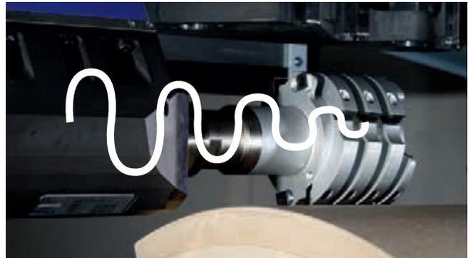
**Liquid cooling and spindle sensor** – liquid-cooled routing spindles with hybrid storage offer a long service life. An additional vibration sensor detects tool unbalances and protects the spindle against overloading, due to high feed speeds for example.
