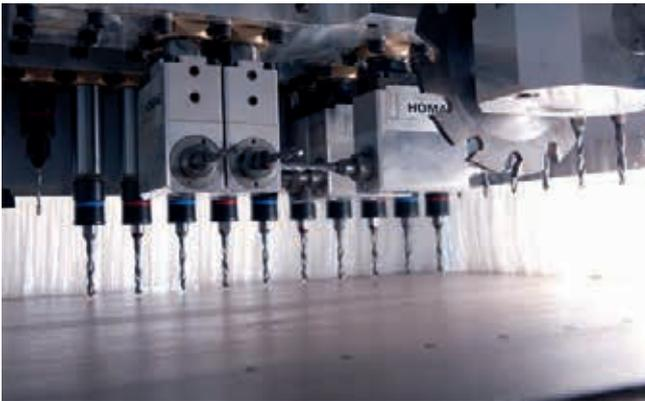
High-speed drilling technology with groove saw
