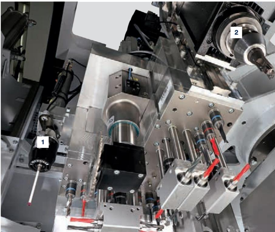
**1** Measuring device to identify the relevant actual dimensions in X, Y, Z with automatic offset correction in the processing program.
