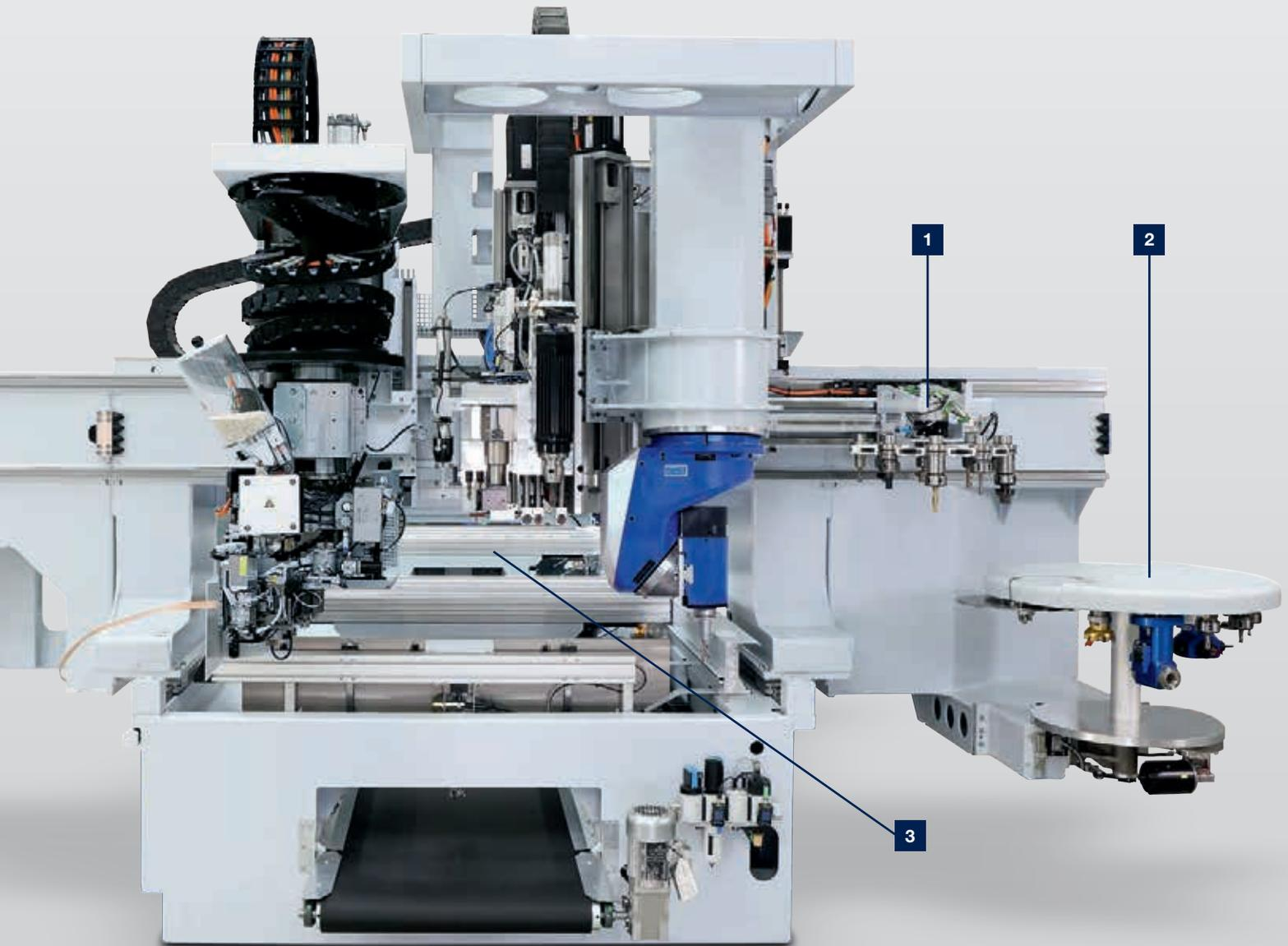
**1** Changers traveling with the spindle for tool change during drilling or edge banding.
