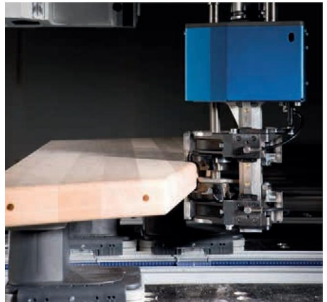
**Pneumatic interface** – the patented interface with 3-way support on all C-axes and 5-axis heads enables the use of traced units, e.g. for precise rounding off at the top and bottom no matter the thickness tolerances.
