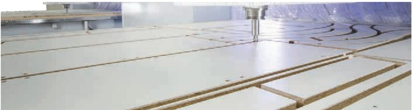
**Nesting processing** of panel materials: waste-optimized cutting to size and processing in the surface
