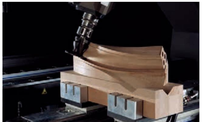
Routing a staircase handrail
