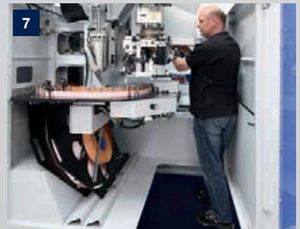
**Easy access** – drill changes, service, refilling adhesive and edge changes can be carried out easily from the front side of the machine.
