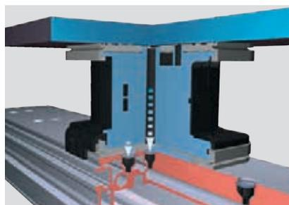
**Dual-circuit vacuum system** – exclusive vacuum clamping technique with double sealing flange for infinitely variable movement of the clamps along the console. The first clamping circuit fixes the clamp on the console and prevents unintentional moving, the second then keeps the material stably in position.
