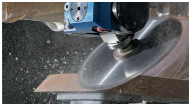
**Sawing, routing, drilling at any angle – FLEX5+ unit** with automatic angle adjustment and automatic tool change. A unique unit for 4-axis spindles, which covers over 90% of 5-axis applications.
