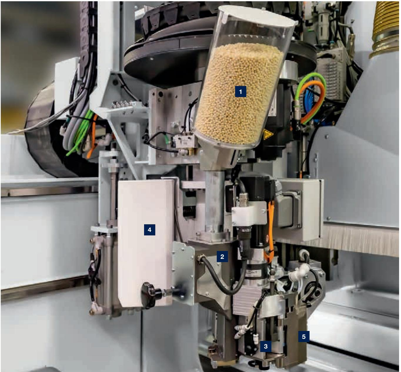
**1 Granulate container:** The granulate container can be released using a bayonet fitting and removed from the machine, meaning that changing the glue color is quick and easy. Alternatively, small amounts can be filled into the application unit directly
