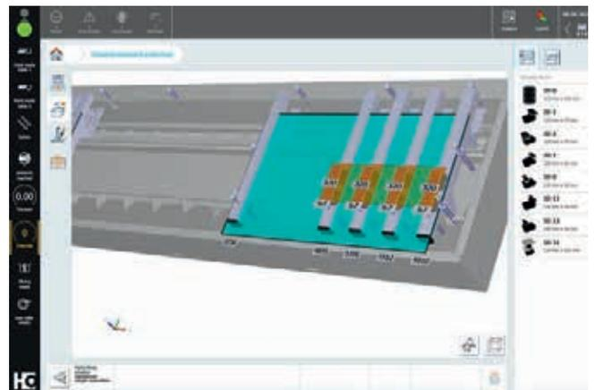
**Automatic suction unit recommendation for workpiece or entire table**
