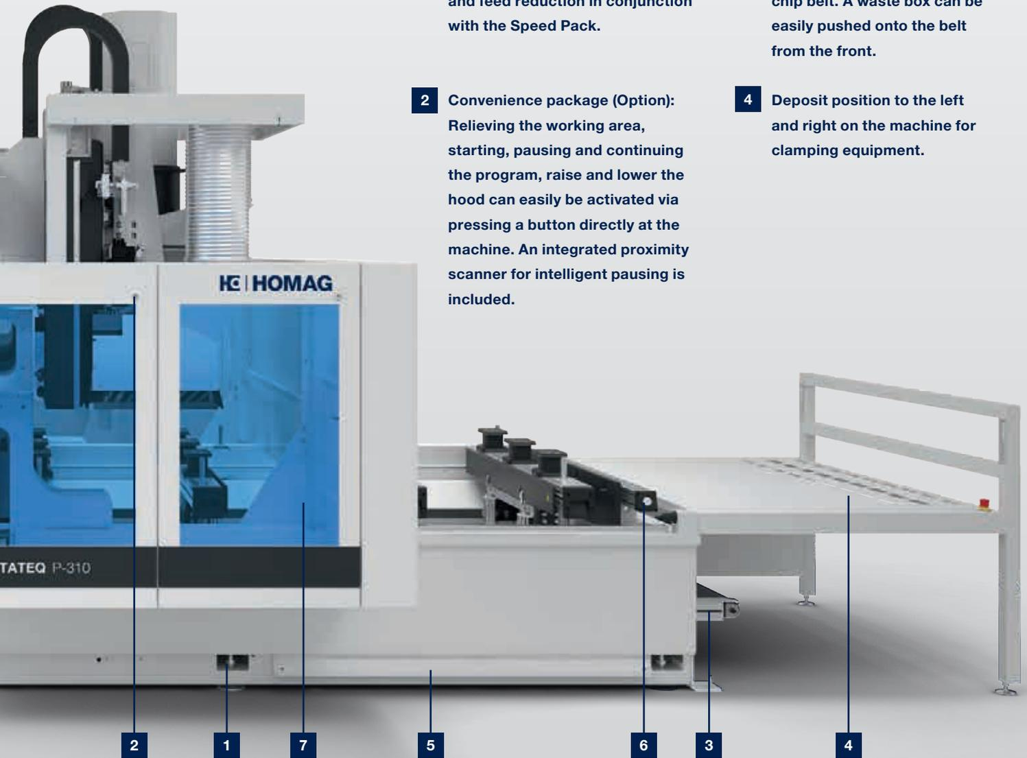
**1 safeScan (Option):** Scanner for contact-free protection of the positioning of the automatic table and feed reduction in conjunction with the Speed Pack.
