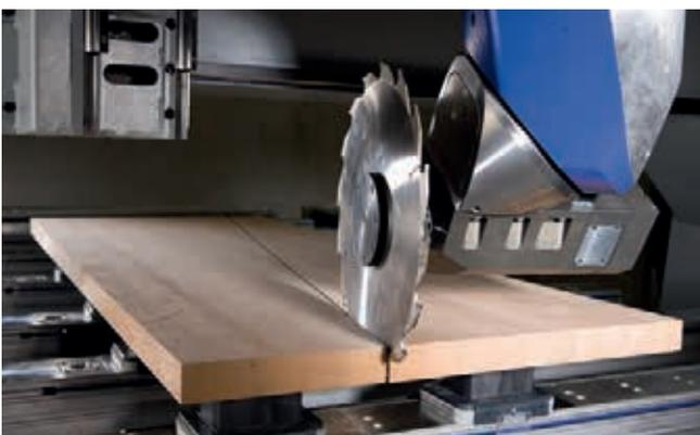
Separating cuts up to 110 mm in height
