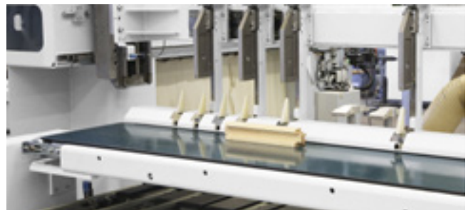
Angular transfer and connection to the hogging machine: Angular transfers and belt transports enable the interlinking with the hogging machine or snipping line.
