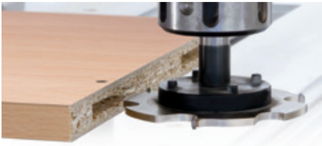
Processing in the workpiece edge area for a wide range of individual connection variations, e.g. for Clamex P connectors
