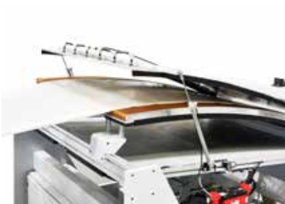
Cooling plate with drying air supply Extraction of the heat from the applied glue film
