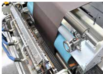
Glue application unit Optimum glue application film thanks to the latest application technology
