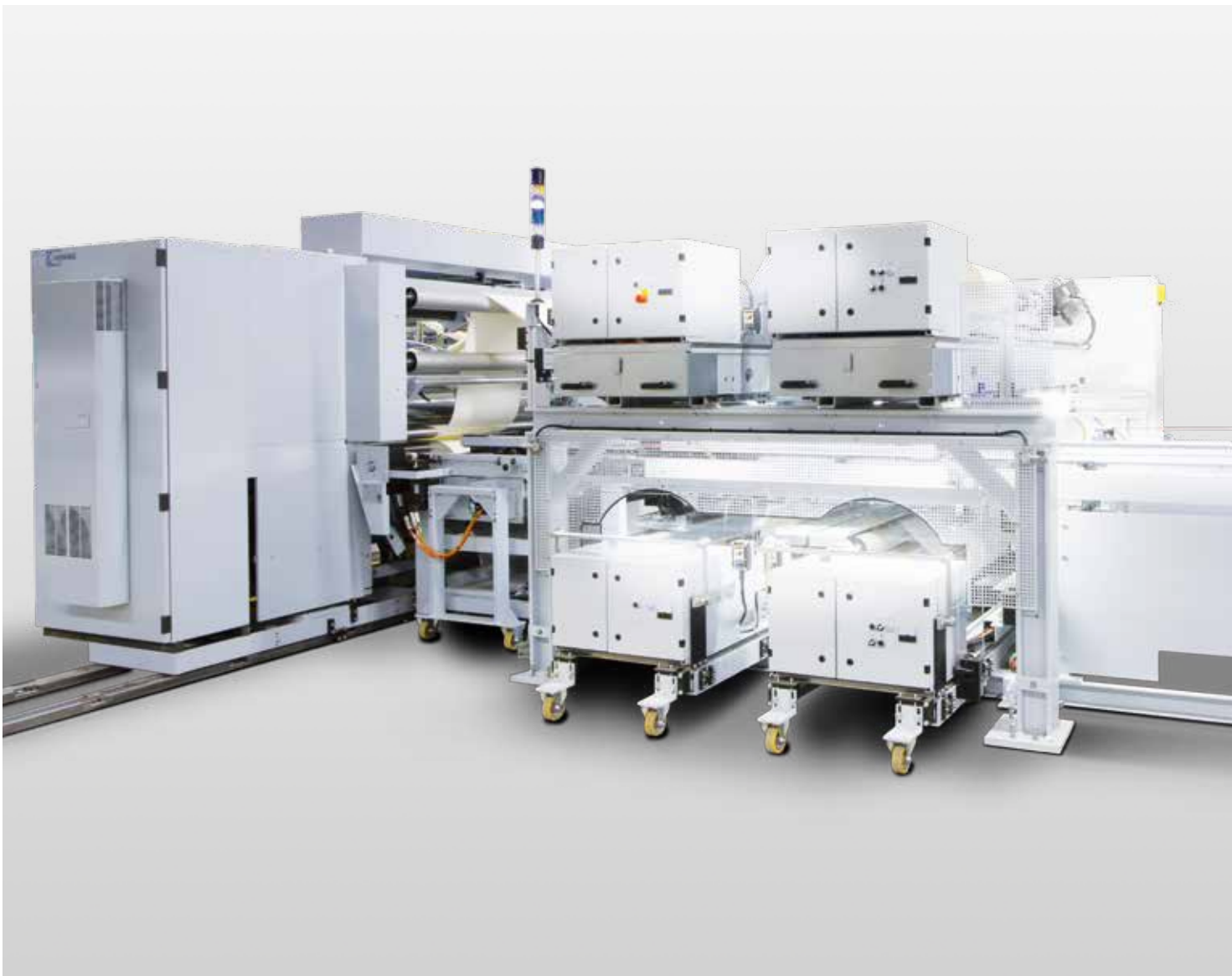
LAMTEQ F-300 laminating line for double-sided coating with the reactTec process.
