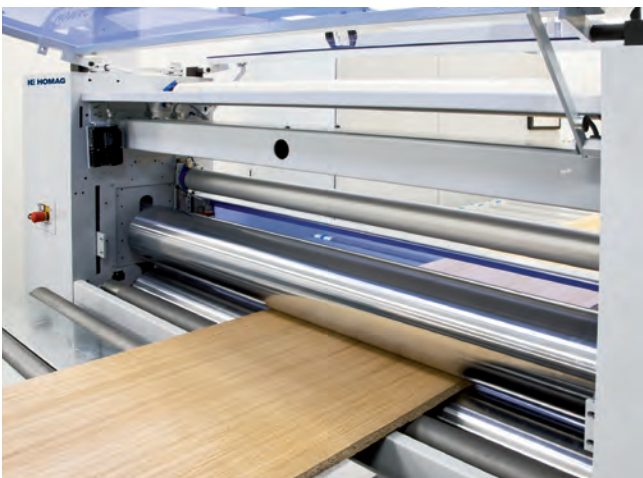
Laminating calender with a pair of rollers for pressing glued workpieces with applied coating materials.
