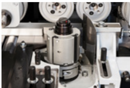
Axial adjustment range up to 75 mm
