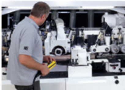
Ergonomic remote control for quick and automatic adjustment of selected spindles
