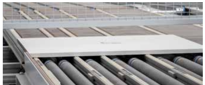
Material transfer from the SORTEQ R-200: Workpieces are forwarded on to the subsequent processing step on an order-by-order basis via transport routes that are connected to the collating center.
