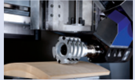
Profiling of shaped components with standard cutter head
