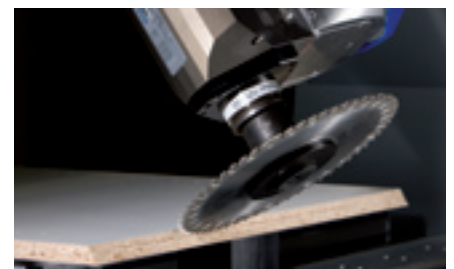
Clean and precise mitre cuts and inclined grooving for a panel connection
