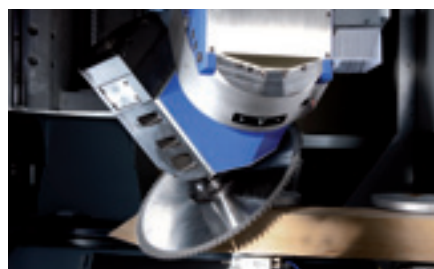
Mitre cut with high cutting depth for frames
