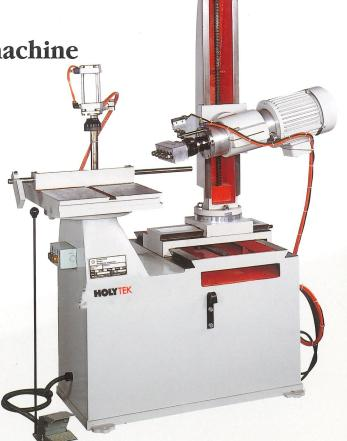
**Horizontal Double Spindle Boring Machine**
