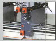
VERTICAL BORING HEAD AND SPEED STABLIZER
