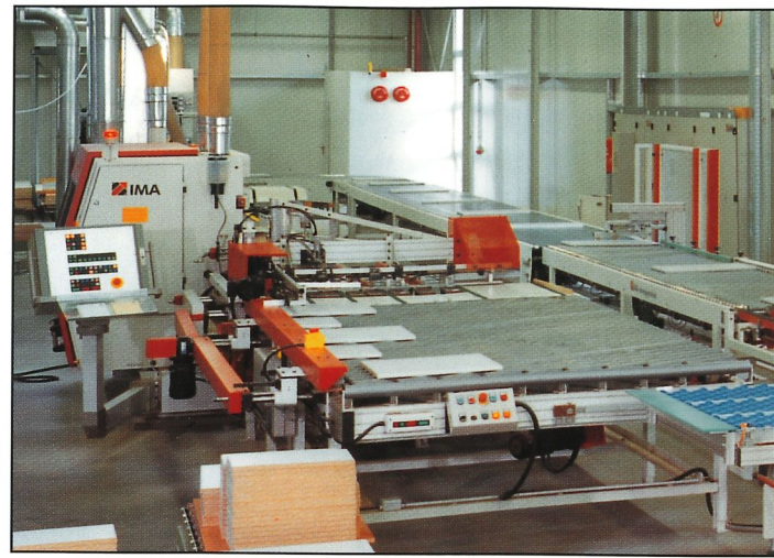
Vacuum infeed table enabling a precise and automatic panel infeed.
