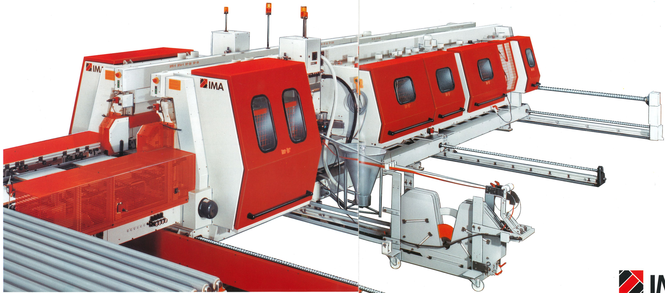
COMBIMA II infeed situation: panel transfer in one plane (optional: 2nd plane).
