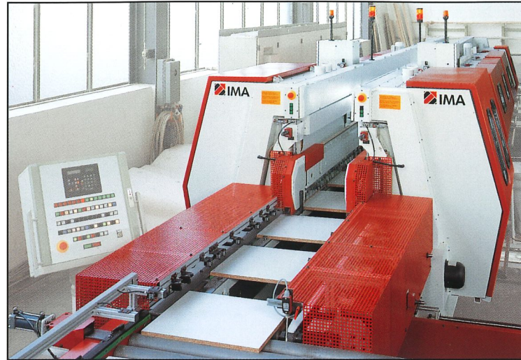
COMBIMA II infeed situation: panel transfer in one plane (optional: 2nd plane).
