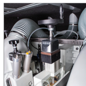
Rail and bearing pad pressure slides eliminate sticking, providing better finish quality and feeding
