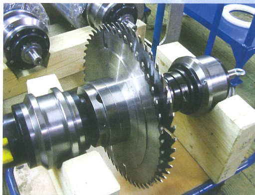
Profil jointer - fernbedienbar Profile jointer - remote controlled
