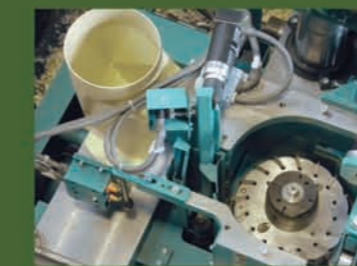
Geradejointer - fernbedienbar Straight jointer - remote controlled
