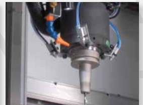
Minimum quantity lubrication, cooling nozzle at working unit
