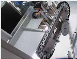
Chain-type tool magazine with 32 places
