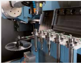
Rake tool magazine with 6 places
