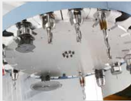
Rotary disk tool magazine with 20 places
