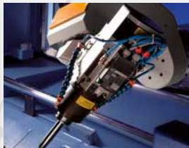
Milling spindle, HSK F63 10 or 15 kW
