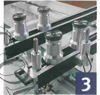
3 Machine table With 8 supporting bars on linear guides
