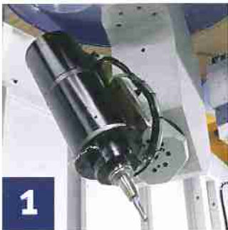
1 Routing unit Standard routing spindle with cardanic suspension, HSK F 63
