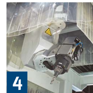
4 Management of waste disposal Swarf collecting basket fixed mounted to working unit
