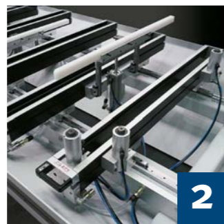
2 Machine table with 8 supporting bars, rapidly adjustable
