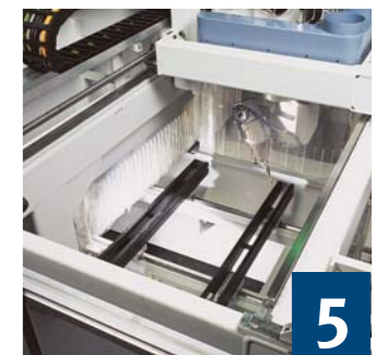
5 Gantry Double guiding system in X axis
