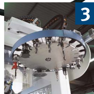
3 Tool magazine Drum-type tool magazine, horizontal, 20 magazine places
