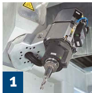
1 Routing unit As standard spindle we offer HSK F 63
