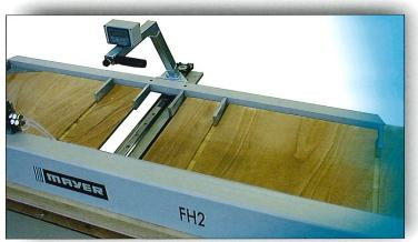
Parallel fence with linear guidance, pneumatic clamping and recessed veneer stops, operating range 20 - 600 mm. The magnetic length measuring system simplifies adjustment by good readability and functions such as absolute/incremental measurement.
