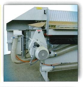
■ The planing unit to recut the edges is raised pneumatically on an extremely precise linear guidance and lowered again when the cut has been completed. This guarantees an optimal cutting result, even for dry and brittle veneers such as oak.
