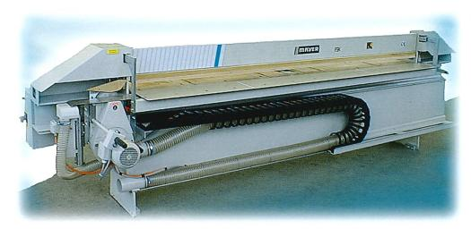
■ The FH2 model is available in 3120, 3520 and 4200 mm cutting lengths. The standard equipment is: saw carriage guided by high-precision linear guidances, planing unit, front supporting table, dust extractor hose for connection to an extraction system, parallel fence with magnetic length measuring system.
