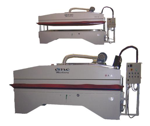
The vacuum press is particularly used for veneer panels wrapping. Using the provided bases, you can have bent panels with plywood foil. The membrane vacuum press is particularly used in the nautical sector and in the high-style furniture industry. According to the type of glue being used, this press can work with or without heating and it has a high capacity vacuum pump. The vacuum press is equipped with a control board which allows all kinds of regulations of the press without any risk.
