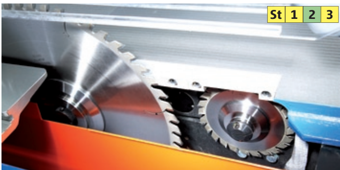
Scoring unit with electronic parking system AUTO-EPS No contamination of scoring saw blade in the parking position, hassle-free installation of main saw blades > 350 mm when scoring saw blade built in.
