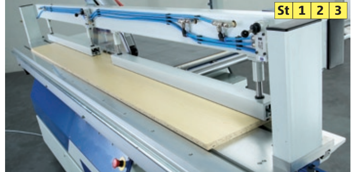
Pressure beam for veneer packages, thin plates, etc.
