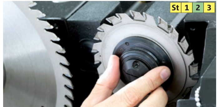
QuickStep scoring saw blade tool-less adjustment of scoring width in 0.05 mm grid system
