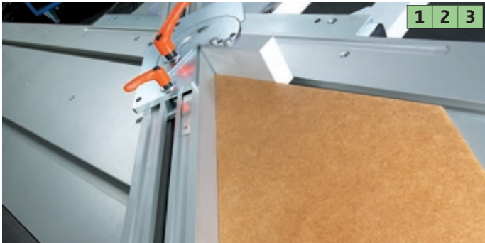
Auxiliary mitre fence the solution to problems when creating pointy and blunt mitres
