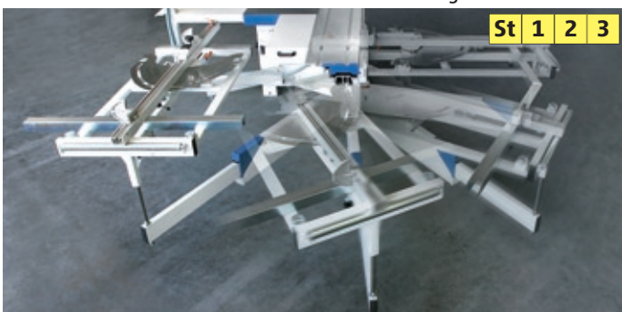
Swing-away device for cross carriages Quick and ergonomic movement to park position
