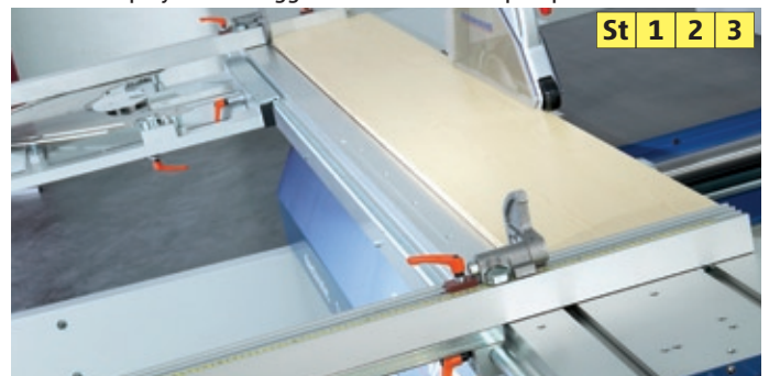
Parallel fence left of the saw blade for cutting long, narrow parts
