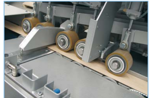
Fig. 42 ... an automatically linked CNC cross-cut system
