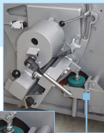
Fig. 12 Height adjustment of saw shaft by an electrically driven lifting spindle
