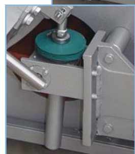
Fig. 12 Height adjustment of saw shaft by an electrically driven lifting spindle
