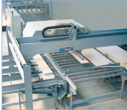
Fig. 35 Vacuum gantry stacker for stacking the strips leaving a K34G/2200 multirip saw with automatic infeed system
