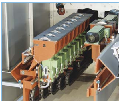
Fig. 34 Lowerable saw heads
