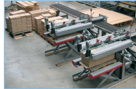
Fig. 37 Length-sorted stacking of cross-cut workpieces on pallets
