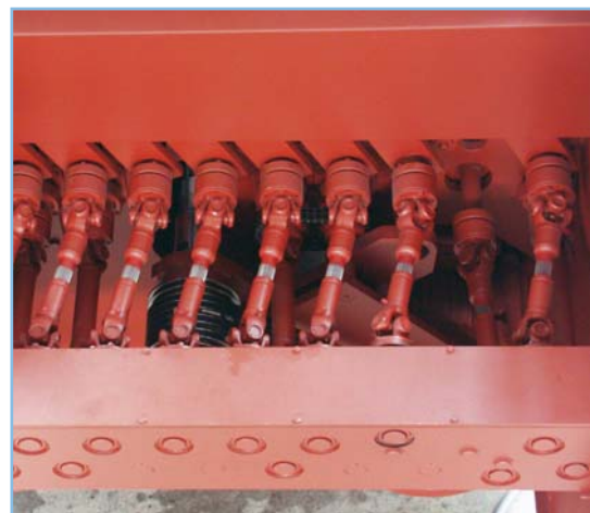
Fig. 20 Drive of feed rollers via cardan shafts
