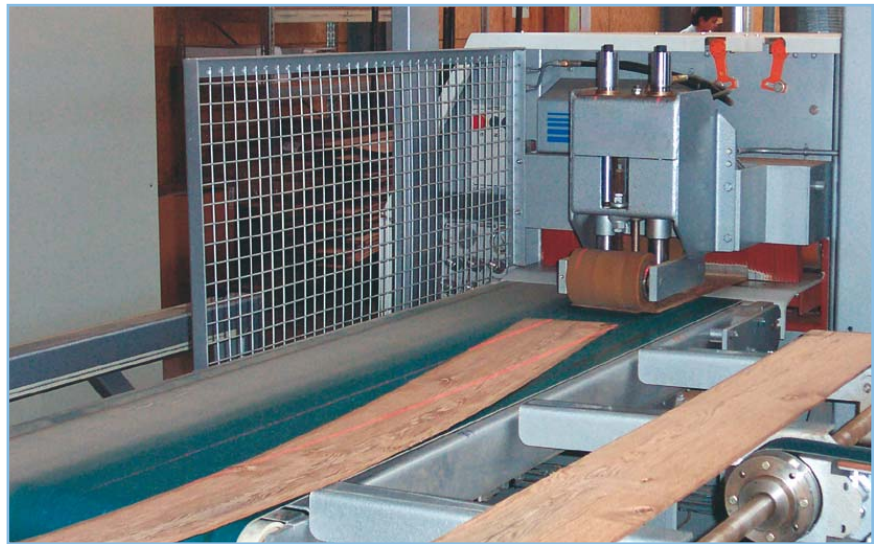
Fig. 41 Rip system used in the production of top layer components of finished parquetry, composed of a K34G/800 multirip saw in special design with moving saw and ...
