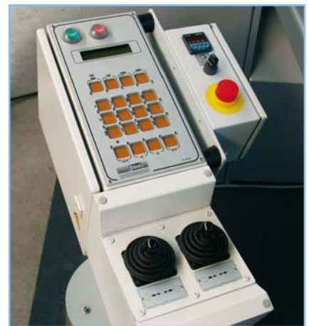
Fig. 20 NCB-2 control with joystick (option)
