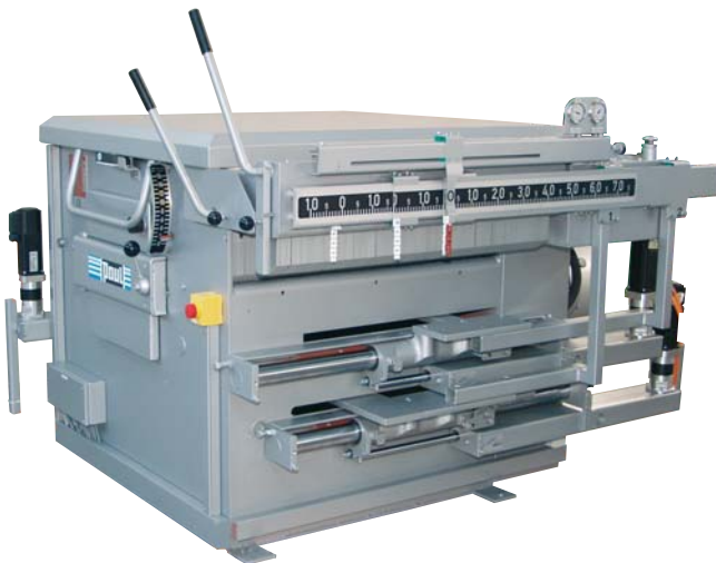
Fig. 5 KME2/1000, saw bushes positioned by a servomotor
