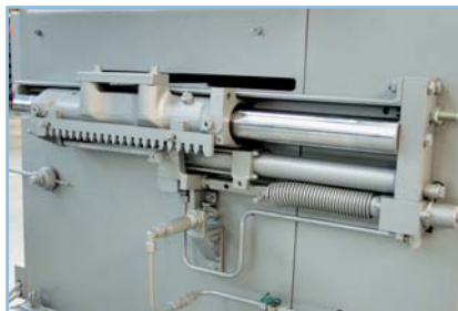
Fig. 16 Hydraulic saw positioning device
