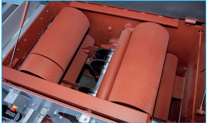
Fig. 10: Fluted feed rollers for improved grip
