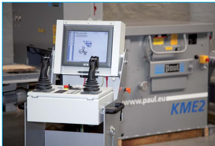
Fig. 23: MAXIRIP operating terminal with touch panel and two joysticks (option)
