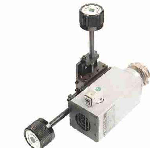
Quick electrical and mechanical release for top and bottom trimmers and corner rounding unit.
