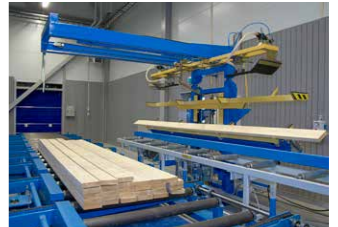
Timber picker with additional roller conveyor system
