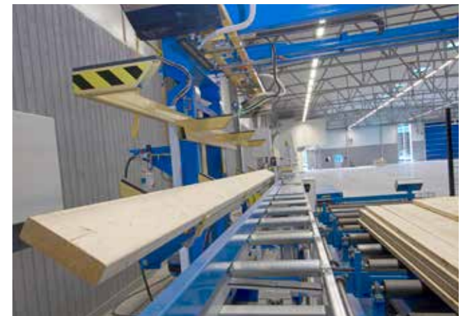
Board is ready to be slid or flipped down to the infeed bench.
