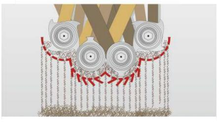
The cutting system comprises of 2 cutting shafts and 2 broaching shafts or optional of 4 cutting shafts.
