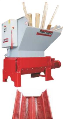
Additional back-up shredders underneath the perforated screen prevent the occurrence of long chips. The radius of the perforation determines the size of the chip.
