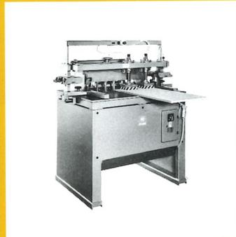
Universal-Dübellochbohrmaschine DB 5Z
