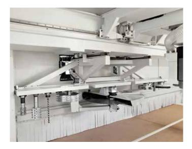
The tool store with up to 12 positions has been designed to have on board all necessary tools to complete the whole work cycle. Dedicated positions for sawblade aggregate of up to 1.020 mm diameter, chainsaw and planning aggregate.
