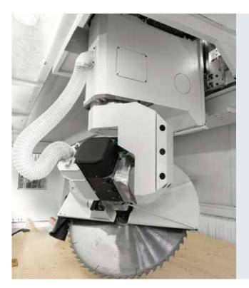
The machining head unit of **Area** has been specially designed to perform, at maximum speed and with perfect quality, all necessary operations to produce construction elements even in the case of heavy duty stock removal.
