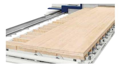
On the highly configurable worktable, handling, positioning and locking of up to 12.700 kg heavy panels are possible fully automatically.
