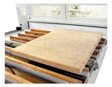
The positioning of bulky and heavy elements might be awkward and difficult; **the laser system simplifies this operation projecting the tool paths on the work piece with precision,** and allowing the operator to centre the program on the piece already loaded on the machine.
