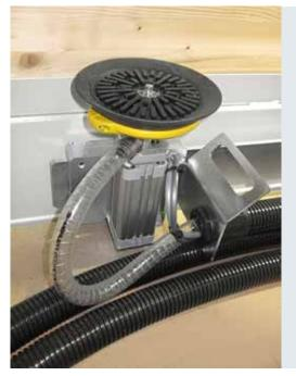
Even small work pieces can be blocked on the worktable thanks to the suction cup system.
