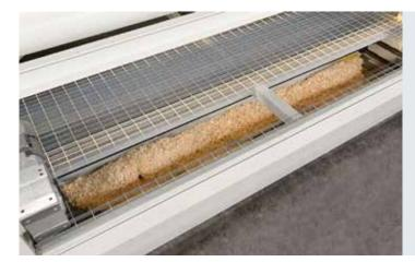
The cleaning systems ensure automatic removal of shavings from under the worktable and on its sides.
