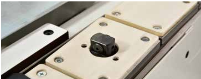
Sliding feed chain from 90 mm for work pieces with minimum width 240 mm. (Dogs pitch between 400 and 800 mm, on request).
