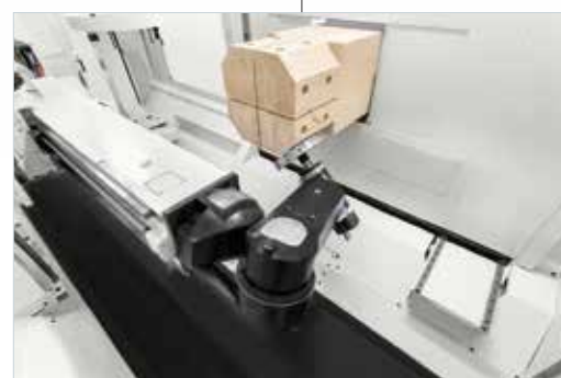
Efficient chip evacuation by means of bi-directional motorized belt, which ensures constant cleaning of the work area.
