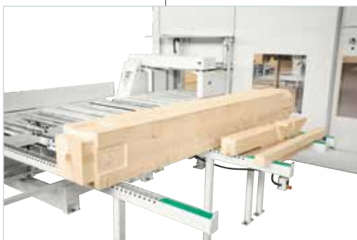
Simple unloading of the finished element by means of a rear mechanical pusher.
