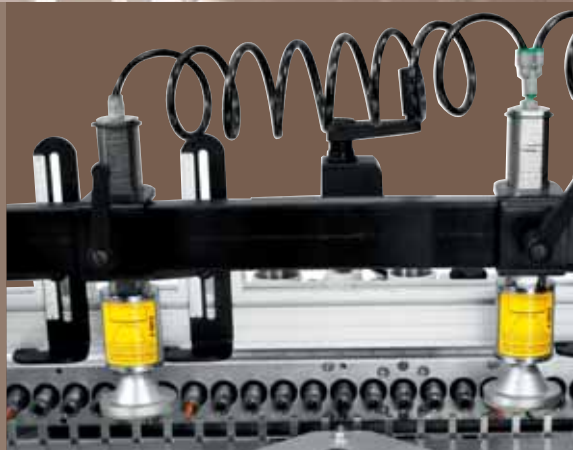
Perfectly aligned joints due to the depth stops with metric rule and work piece locking pistons
