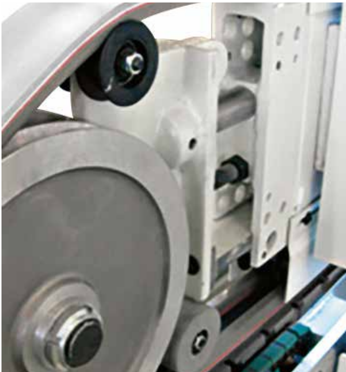
Top pressure belt, with automatic vertical movement by HMI depending on the panel thickness.
