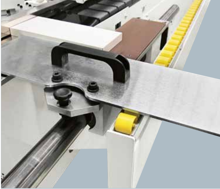
Maximum machining precision even with narrow panels / drawers thanks to the manual infeed device (opt).
