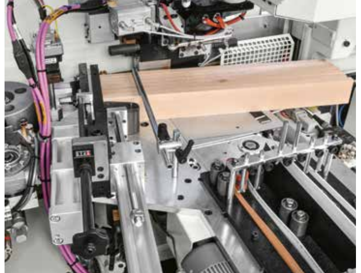
Quick and easy processing of solid wood lipping up to 22 mm thick, even when the 2- or 6-edge roll magazine is installed.
