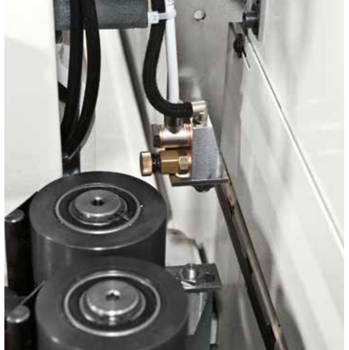
Liquid to cool the temperature of the glue in the area exceeding the edge, in order to keep the tools clean for the subsequent processing (opt.).
