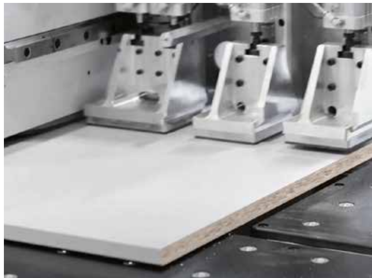
Maximum grip of the panel thanks to top and bottom grippers and frontal stop.
