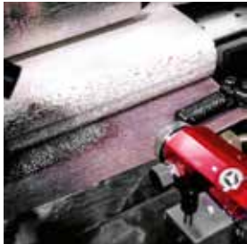
Station for glue application on a non-flat surface
