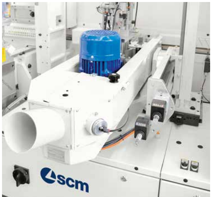
Sanding units for the finishing of doors machined with veneer edge.
