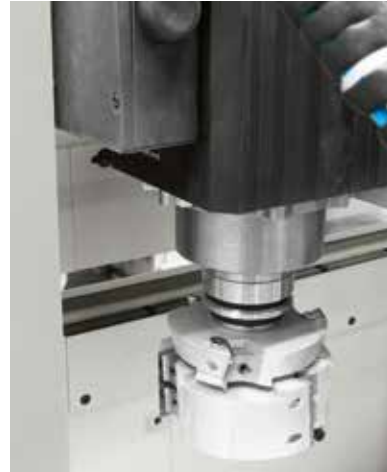
MX80 HSK SOFT profiling unit with quick tool change.
