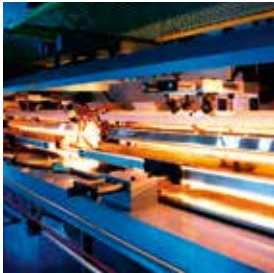
Station for laminate softening
