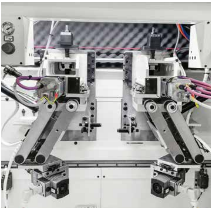
C3 rounding unit specific for the finishing of corners on three or four sides of the door.
