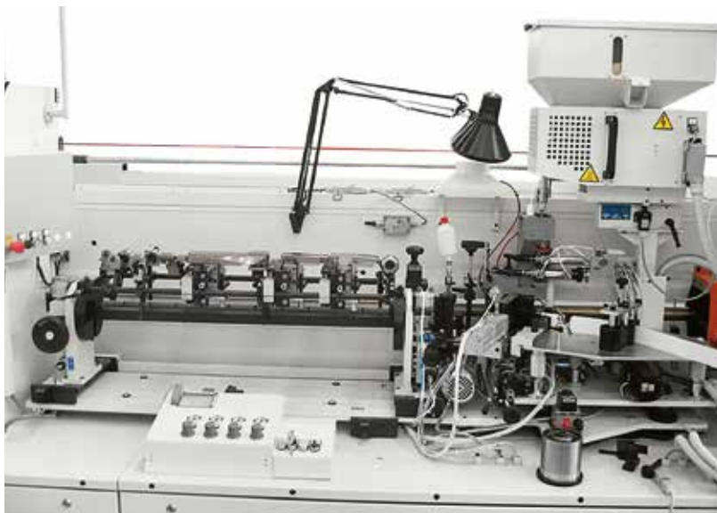
Gluing unit for the processing of doors with thin/soft edges.
