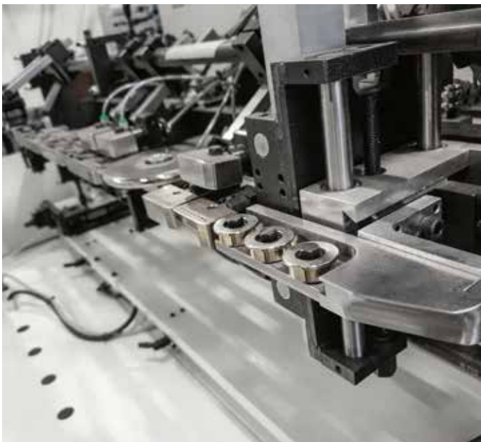
Pads specifically shaped for every single profile.
