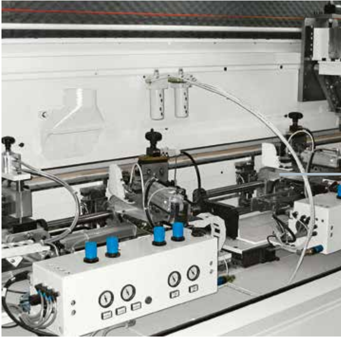
Corner finishing units for doors edgebanded on 3 or 4 sides.
