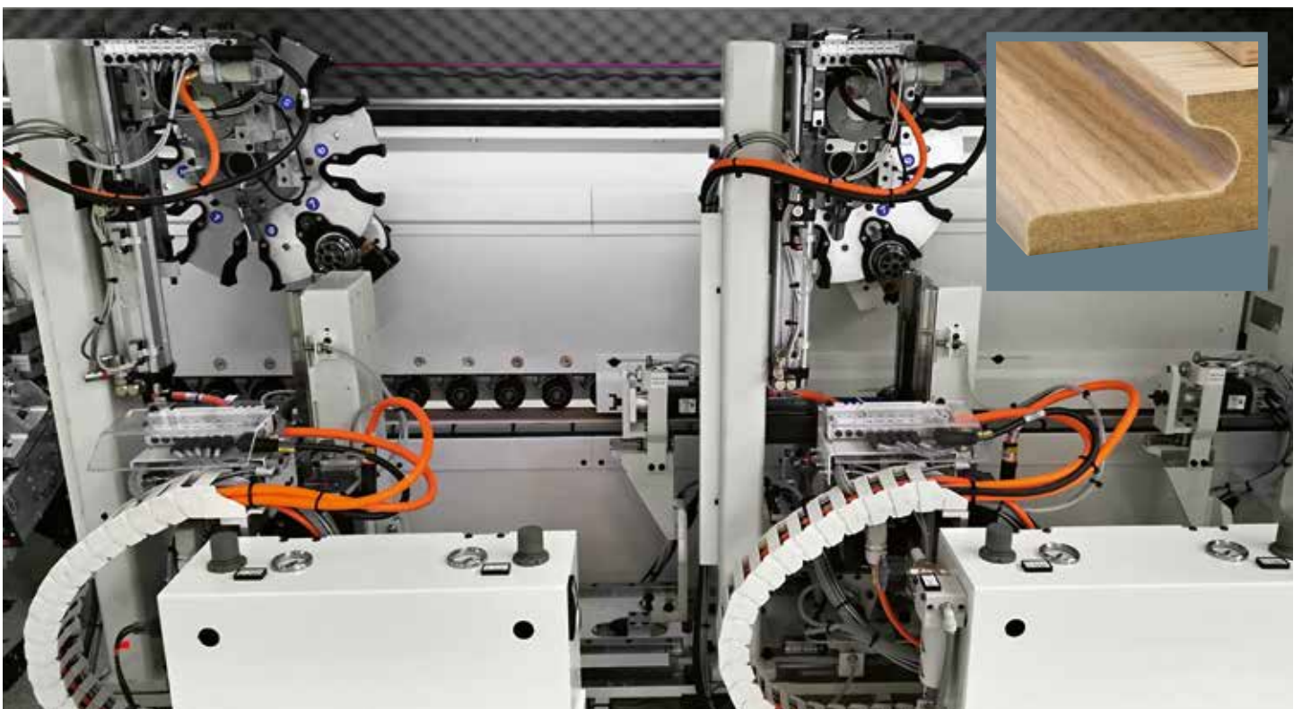
2-motor corner rounding unit, power assisted, for the complete finishing of "J" and "C" profiles with the special J-side kit.
