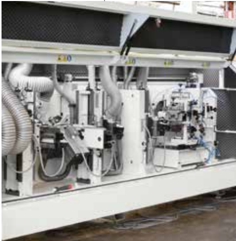
Profiling area with very high performance motors for maximum precision.
