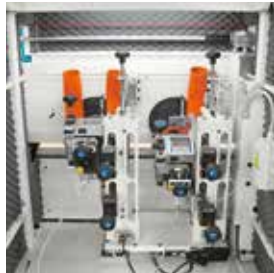
Station for laminate finishing
