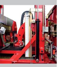
Hydraulic lifting mechanism and precise height adjusting because of the scale.
