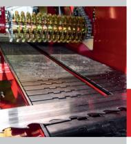
The cutting height of the 80mm wide blades is between a minimum of 7 and maximum of 420 millimeters. Professional and worldwide proven sawing technology is used.
