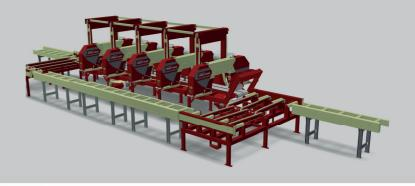
Rollers and conveyor chains are hydraulically driven: Uncompromising even at the heaviest hard-Lumber can not slip.
