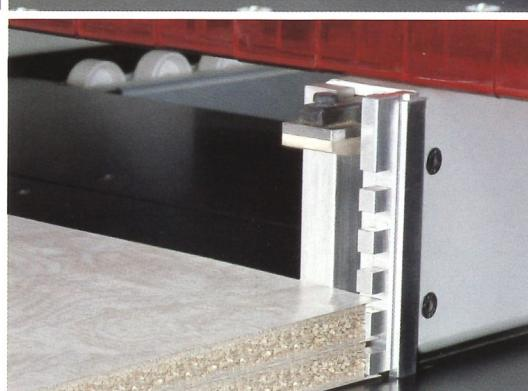
Finger system for cutting panels, even in stacks with overhanging edges. The fast replacement of fingers is ensured by a Selco patented system.
