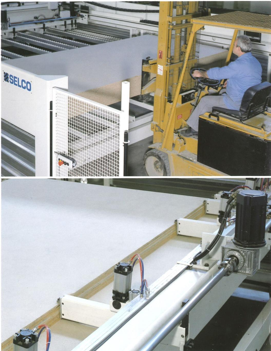
Special floating and self-levelling grippers with lower retractable fingers allow a fast taking over of the stack.
