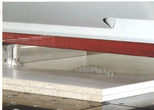
Electronic adjustment of scoring saw blade by means of the Digiset device. This system is used to memorize and recall the aligning positions of 10 saw blade sets, thus making extremely fast and precise the saw blade adjustment.
