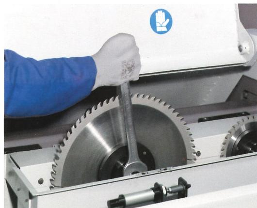
The fast and safe saw blade change is made by using a single wrench.
