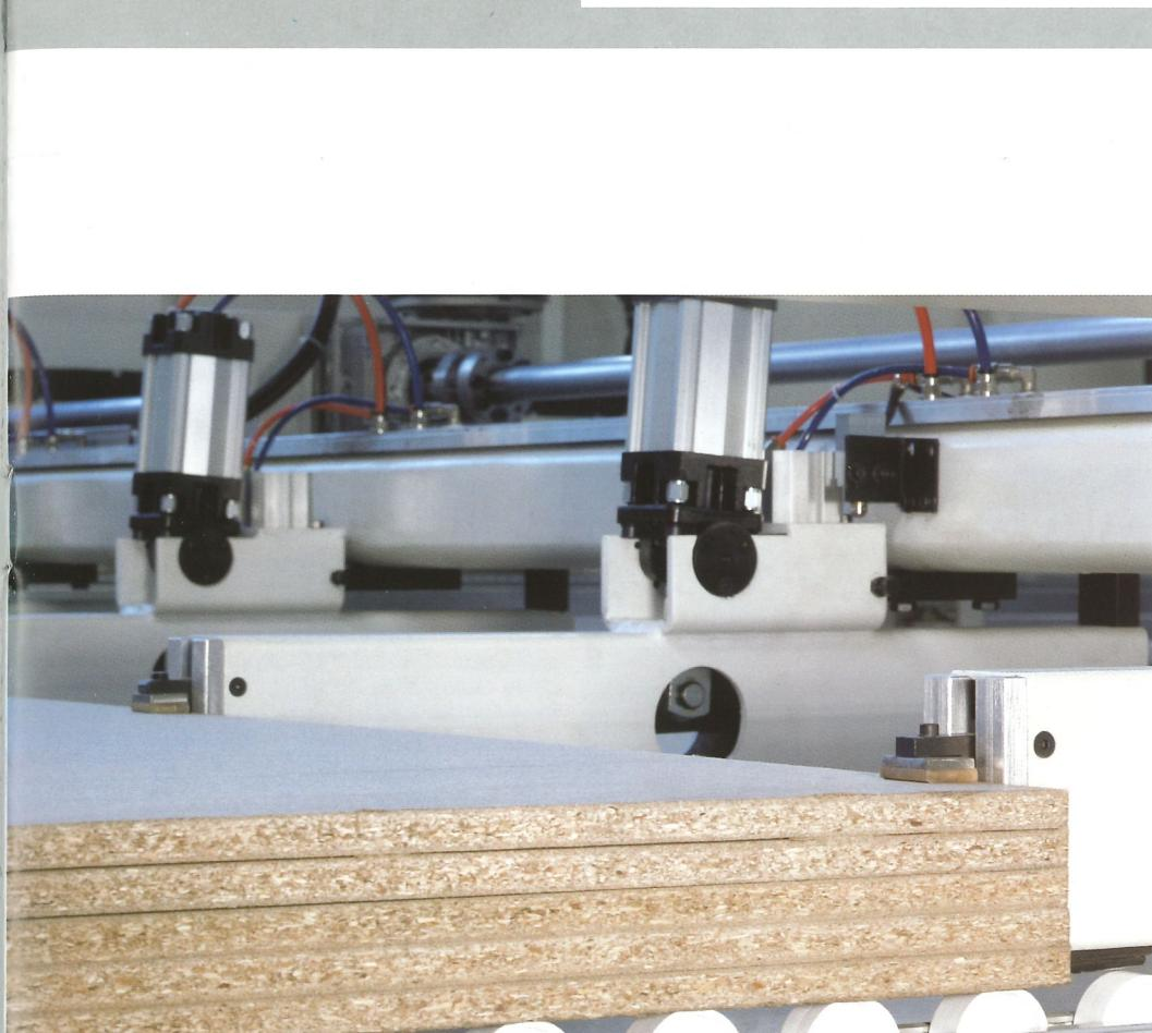
Robust front aligning devices align the stack of panels against the pusher grippers.
