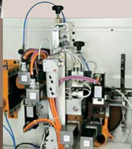
Multifunctional edgescraping unit
