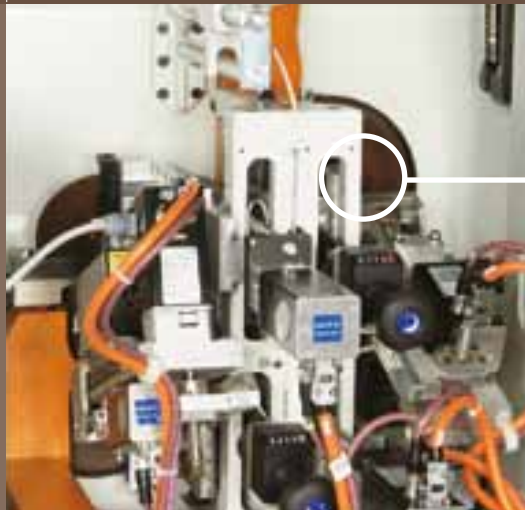
Multifunctional fine trimming unit
